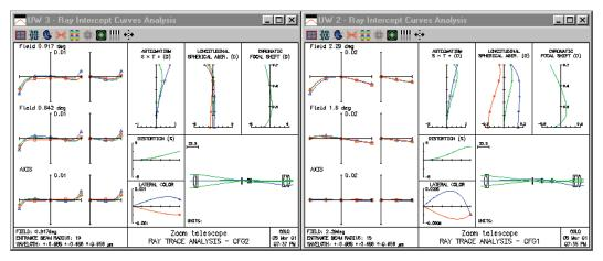
OSLO has a number of routines to simplify working with zoom systems. The aberrations toolbar in the text output window contains several buttons dedicated to zoom systems, permitting analysis of a system in several positions with single commands, for example:
